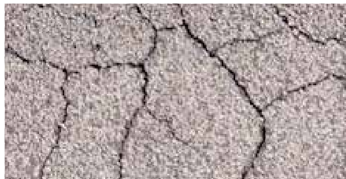
SBS modified shingles resist cracking and shrinking in both hot and cold weather climates.
